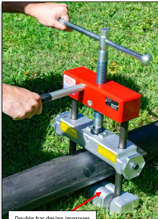
Double bar design improves the quality of flow control
